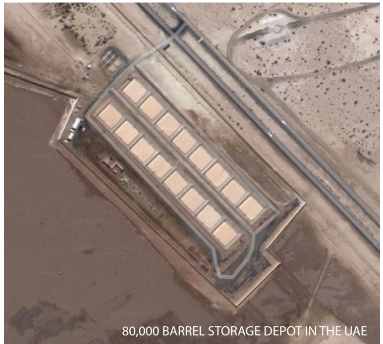
ROUNDED CORNERS REDUCE RISK OF LEAKAGE
